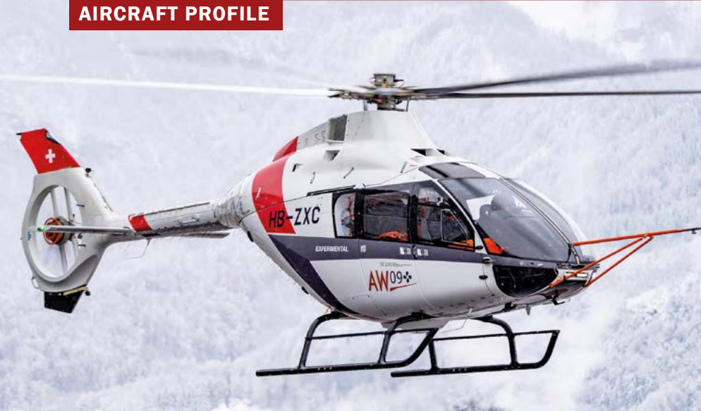
The design of the AW09 continues to evolve, with recent testing revealing reshaped upper cowlings that improve the aircraft's aerodynamics. (Photo: Thomas Frevillier)
