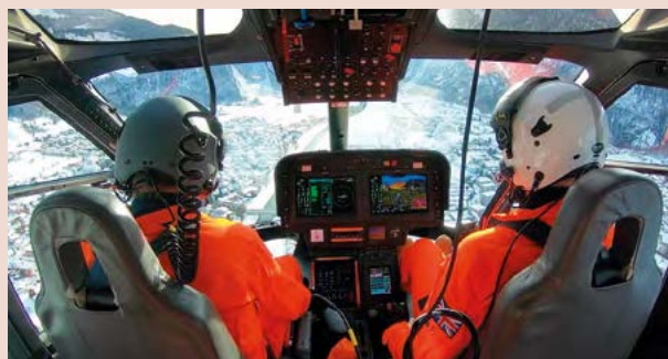
The third prototype was fitted with Garmin's G3000H avionics suite towards the end of 2020. (Photo: Kopter)
